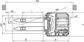
Ast = Wa + x + I6 + aAst = Working aisle width with load l6 = Pallet length (800 or 1000 mm)
